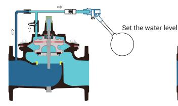
Water low  $\rightarrow$  pilot valve opens  $\rightarrow$  main valve drains  $\rightarrow$  main valve opens.
