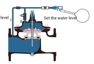
Water reaches pilot valve level  $\rightarrow$  valve closes  $\rightarrow$  water fills bonnet chamber  $\rightarrow$  main valve closes.
