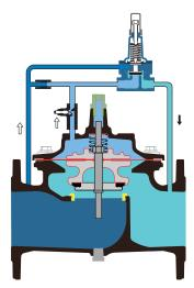
When the upstream pressure drops below the pilot valve's set pressure, the pilot valve closes, allowing water to enter the upper bonnet chamber of the main valve and forcing the main valve to shut.
