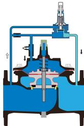
When the upstream pressure exceeds the pilot valve's set pressure, the pilot valve opens, allowing the upper bonnet chamber of the main valve to drain and enabling the main valve to open.
